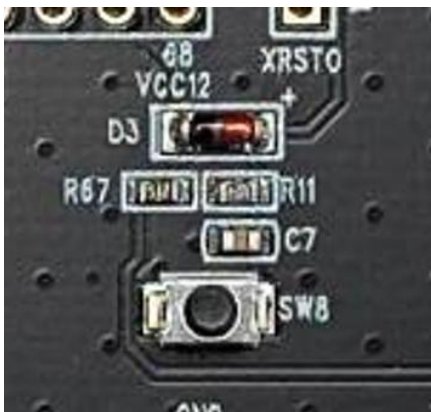
SW8 Reset button, low active
